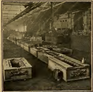
Fig. 64. Completing Moulds Ready for Pouring.
